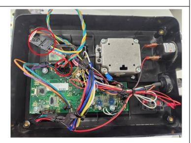
11. Connect the 8-pin connector from the Operator Sensor and the 12-pin connector from the OverWatch harness into the ECU.
