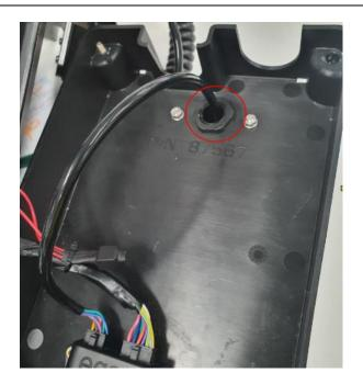
8. Pull the operator sensor cable tight and secure the cable to the large hole in the base of the operator sensor mounting bracket by using a cable tie.
