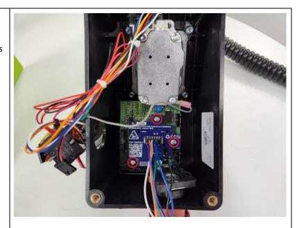
11. Install the Overwatch joystick connectors in between the joystick and the control box circuit board.
